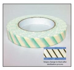
Lead free or Lead/Latex autoclave tape is available for purchase through eShop (Fisher Scientific catalog # 19-305-245 respectively). This tape clearly indicates that it is lead free. It has green lines that turn dark after 15 minutes of exposure to a temperature of 121°C (250°F) in a steam autoclave.
