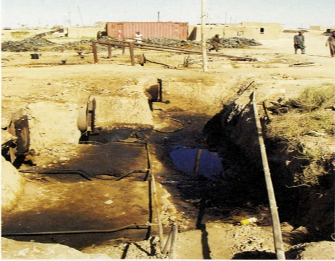
Boilers leaking crude oil onto the ground at Shiburghan
