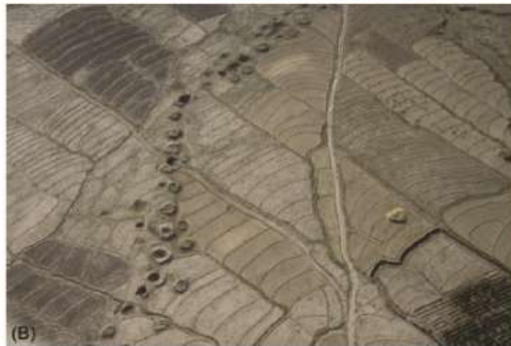
FIG. 3.31. (A) Photograph of karez cleanout shafts along valley floor. Karez along irrigation canal or ephemeral or perennial rivers can take advantage of leaky canals and infiltration from nearby losing or infiltrating streams to gain shallow ground-water recharge (Photograph by L. Sinfield, 2012). (B) Photograph of multiple generations of karez cleanout shafts showing filled and abandoned portions, together with more recent open shafts (Photograph by U.S. military).
